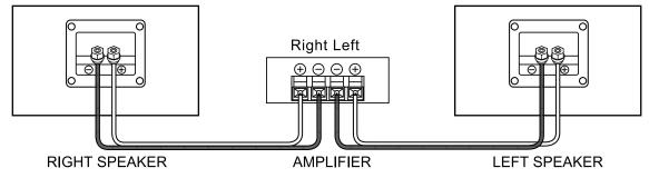
If the polarities of left and right are not aligned properly, the quality of the reproduced sound, the ambience and the feeling of direction will be markedly impaired.
